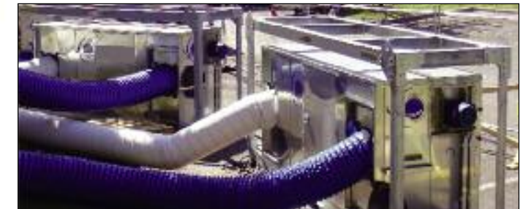
Wet side, MS-6000/5000 pulls moisture from ambient air.
